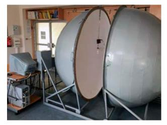
Figure 3. The measuring station for measuring the luminous flux
