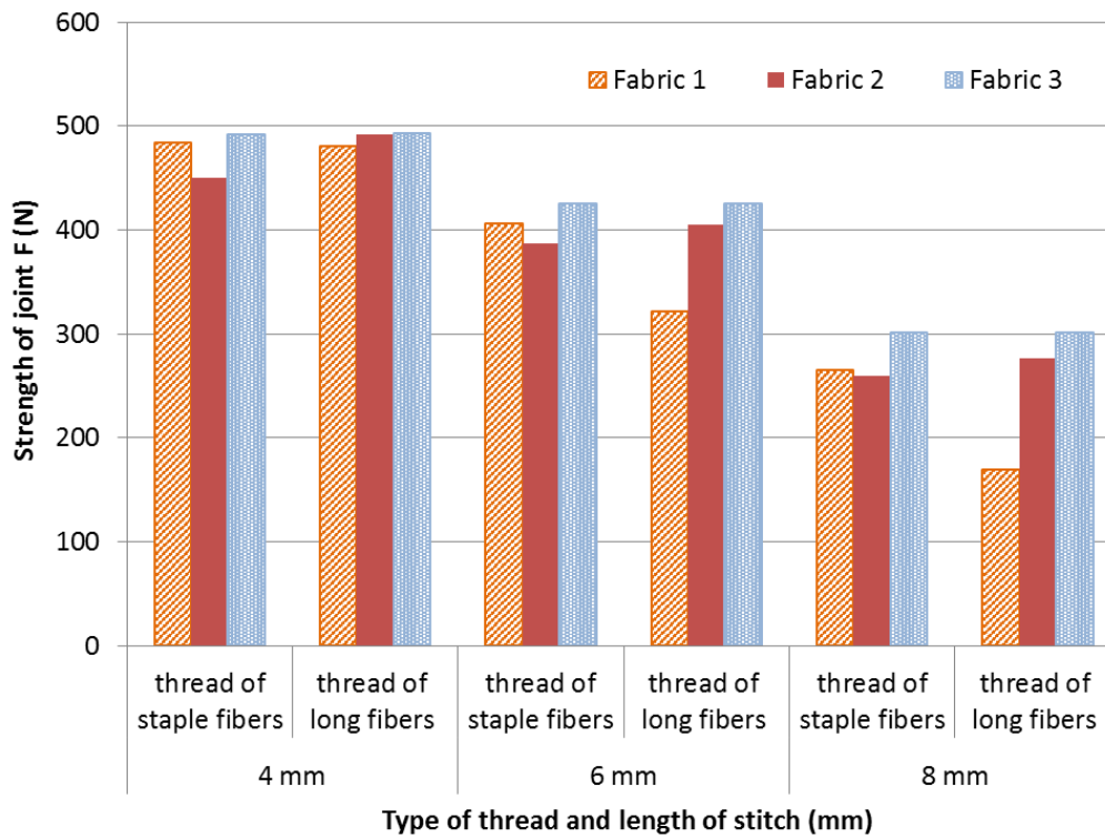
Figure 3. The change of the strength of stitched joints, stitched in the weft direction.
