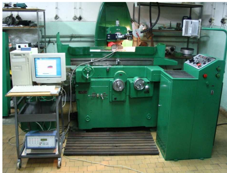
Fig. 1. Experimental setup for monitoring of the surface grinding process (overall view)
