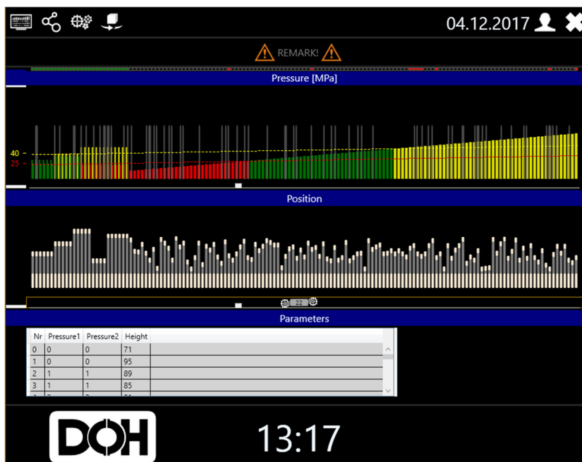
Fig. 7. The visualization system for the entire longwall with a visible shearer
