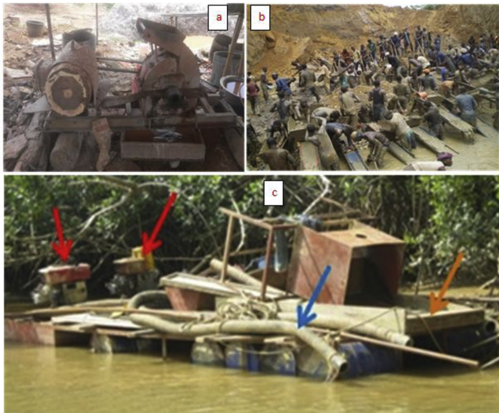
Fig. 1 – Artisanal Small Scale Mining Methods: (a) Changfa in Operation, (b) “More Blade” Method, and (c) Typical Dredge Method: Changfa motors (arrowed red), suction hose (arrowed blue) and working platform (arrowed dark orange).
