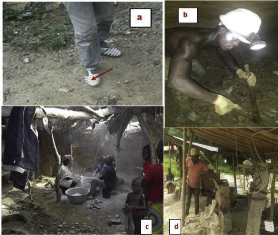
Fig. 6 – Some safety conditions in small scale mining in Ghana: (a) Miner going underground in rubber sandals, (b) Much equipped miner breaks rocks using pickaxe, (c) Dust from sieving milled ore, and (d) Changfa operators without PPE.
