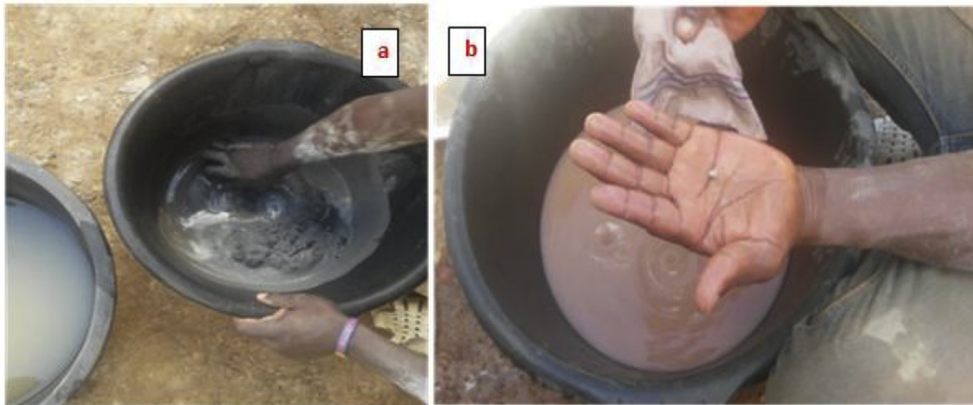
Fig. 8 – (a) Miner stirs slurry with bare hands, (b) Miner holds mercury-gold amalgam in the palm.
