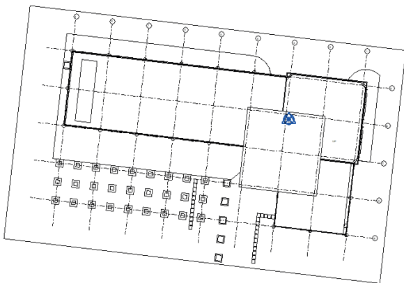
Fig. 4. Third floor plan with orientation set relative to True North in Revit
