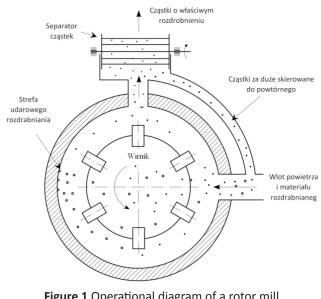
Figure 1 Operational diagram of a rotor mill with particle separation
