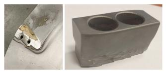
Figure 4 View of the rotor mill's working components after 60 hours of operation (micronised material – oat seed coats, humidity <8%)
