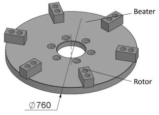
Figure 2 Working components – beaters and rotor
