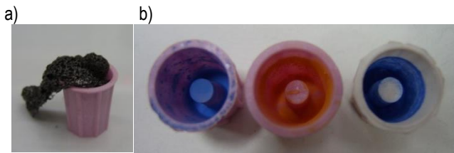
Fig. 9. View of the crucibles after derivatograph tests, remnants of: a) PC, b) B, c) O, d) G
