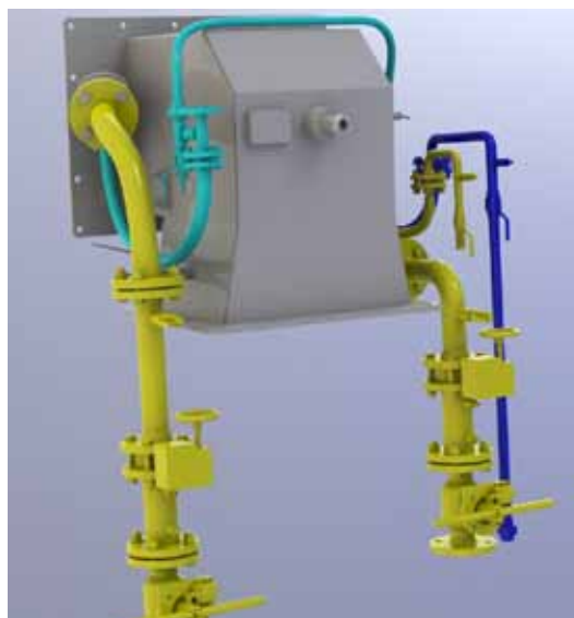
Fig. 2. 3D visualization of the HTB burner with burner piping
