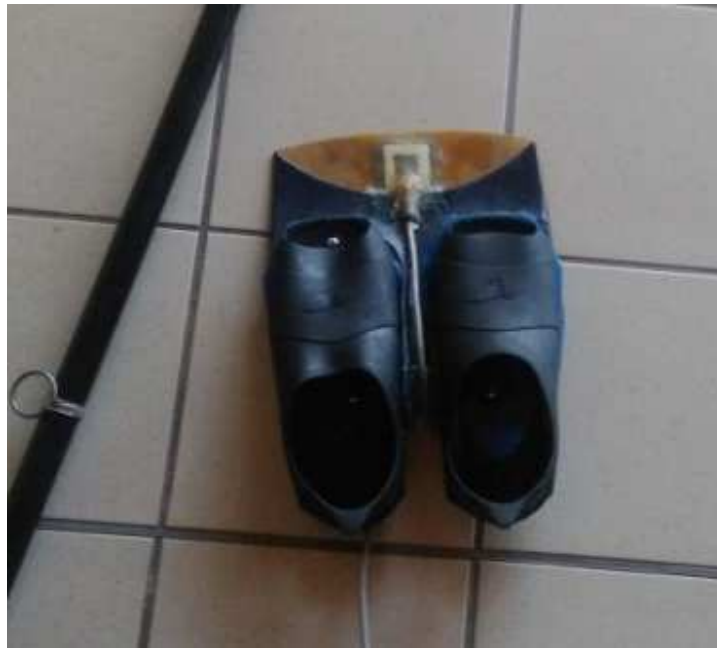
Fig. 1 The testing device - Prototype of monofin with plate cut at the toe line and equipped with strain gauges.
