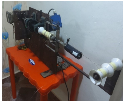
Foto 2. Machine Set up as a Spinning Machine
