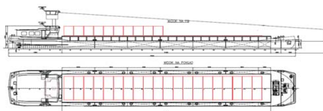
Figure 2. General arrangement plan of the motor cargo vessel BMN 700
