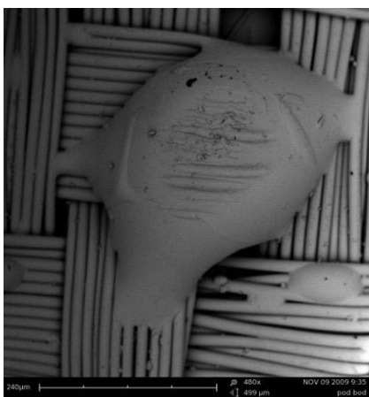
Figure 3. Polymer dot on lining created during the coating process.
