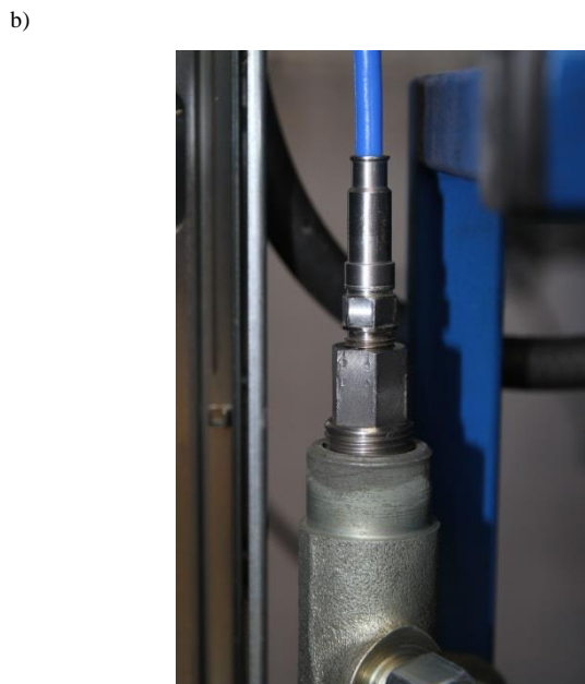
Fig. 1. STPiW-2 testing table: a) general view, b) AVL SL31D2000 pressure sensor fitted in the adapter: 1 – fuel injector tester, 2 – high-pressure pump tester, 3 – testing table control module, 4 – injectors, 5 – fuel dose measurements cylinders, 6 – high-pressure pump, 7 – overflow measurement cylinders
