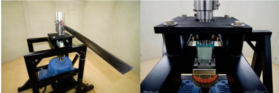
Fig. 3. The Whirl Tower Test Chamber and Test Stand [8].
