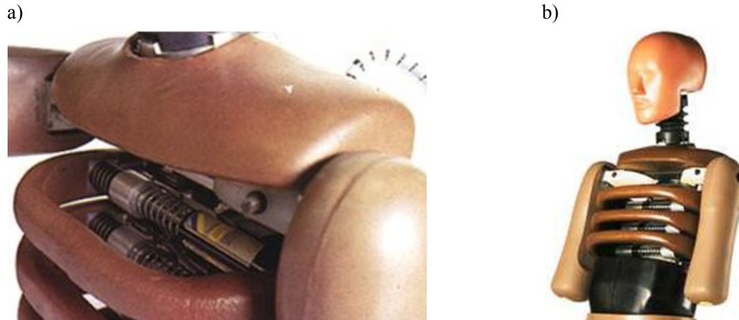
Fig. 4. Hybrid III Dummy: a) chest, b) view of a whole chest [9]
