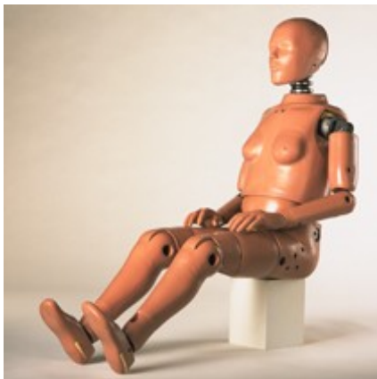
Fig. 6. Dummy of a 5 centile woman of Hybrid III [14]
