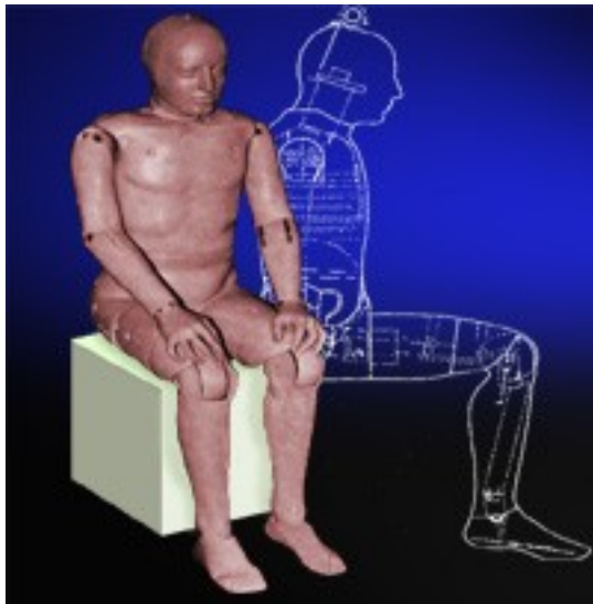
Fig. 2. Hybrid II dummy of a 50 centile man [4]
