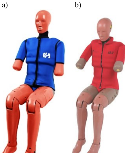
Fig. 13. EuroSID-2 dummy: a) male, b) female dummy [27]
