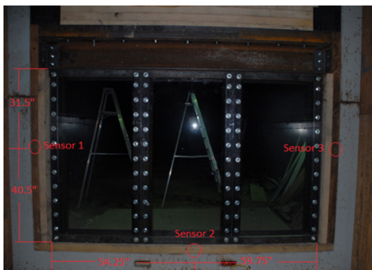
Fig. 3. Pressure Sensor Locations for Half-Width Scale Testing
