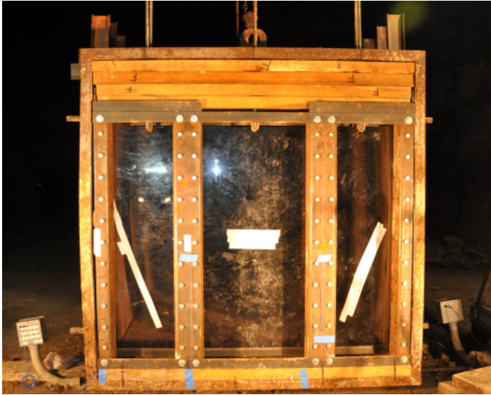
Fig. 9. Quarter-Width Scale Polycarbonate Wall System
