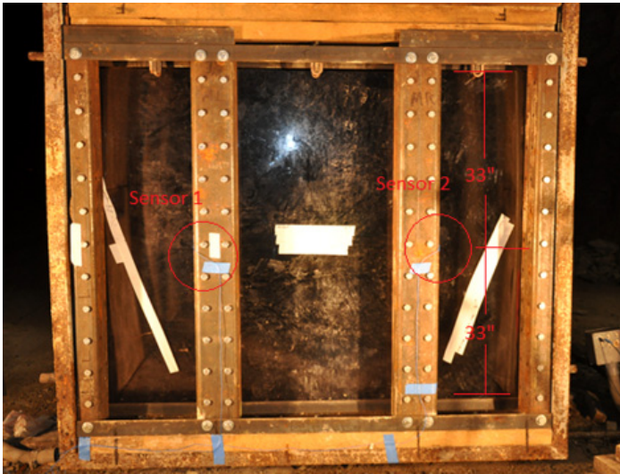
Fig. 10. Sensor Placement for Quarter-Width Scale Testing
