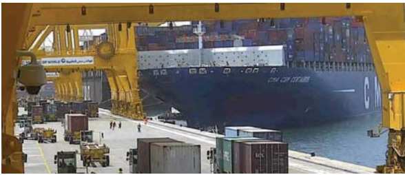
Figure 5. CMA CGM Centaurus making contact with the quay (MAIB, 2018)
