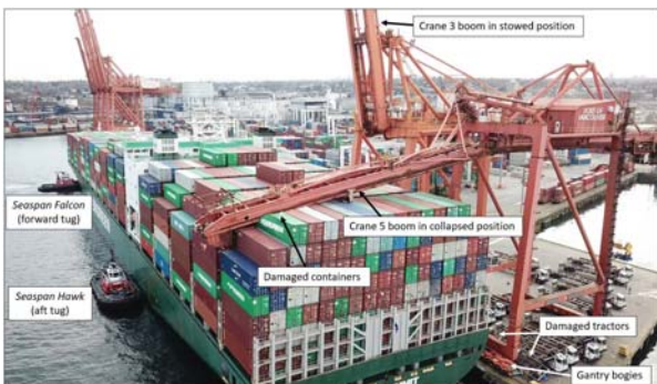
Figure 6. Striking of berth and shore gantry crane with Ever Summit (TSB, 2020)
