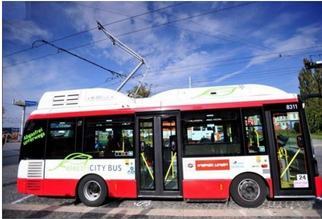
Fig. 7: Electric bus charged from the trolleybus overhead line (the city of Pardubice).
