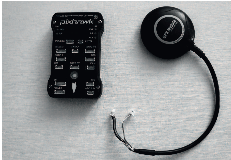
Figure 1. The Pixhawk v2 flight controller with Neo-M8N GPS with Compass GNSS receiver
