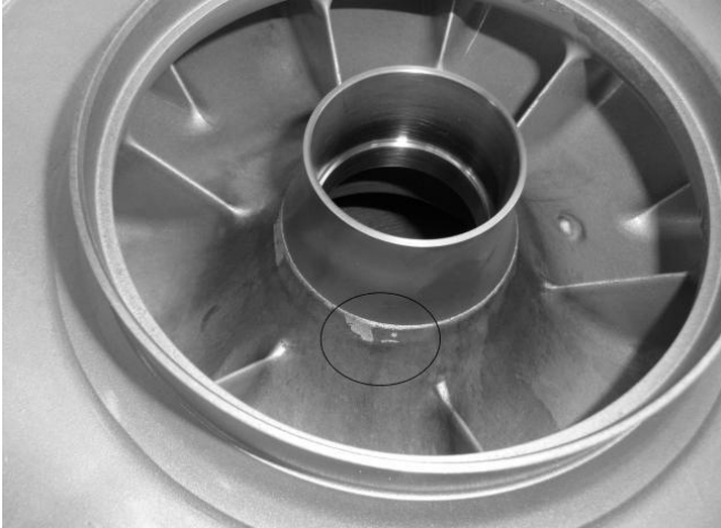
Fig. 3. View of a damage to the walls of flow channel near the steering compressor set (photo P. Rutkowski)
