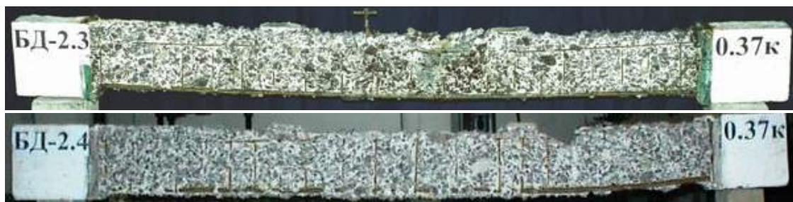
Fig. 6. The overall view of failure of experiment beams of level 0,37M max
