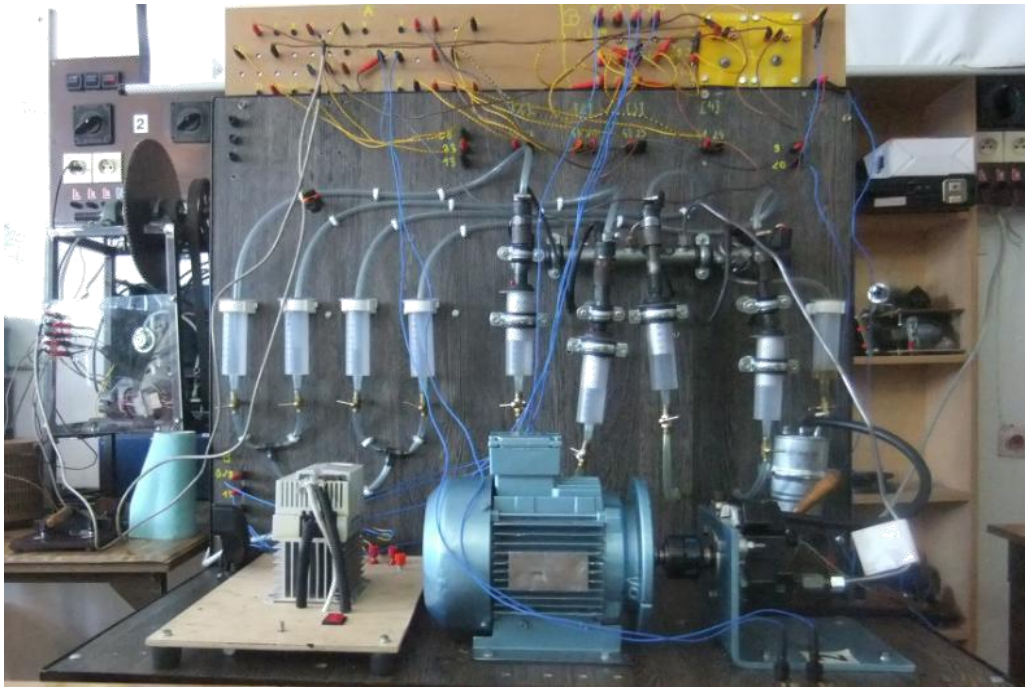
Fig. 7. Test bench for simulating the work of the EDC system
