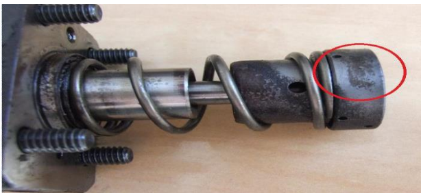
Fig.1. Damage to the pressure section – uneven wear
