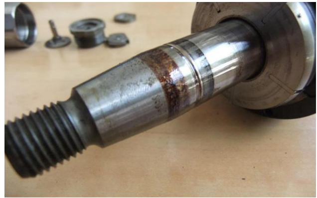
Fig.3. Damage to the shaft – grooves visible
