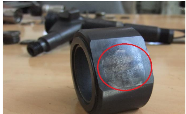
Fig.4. Surface damage to the roller – deformation visible
