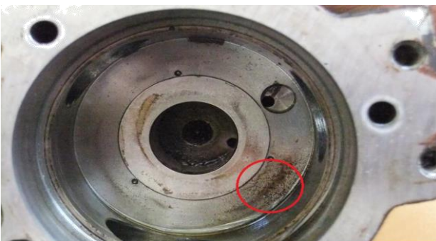
Fig.2. Damage to the pump housing – indentation visible
