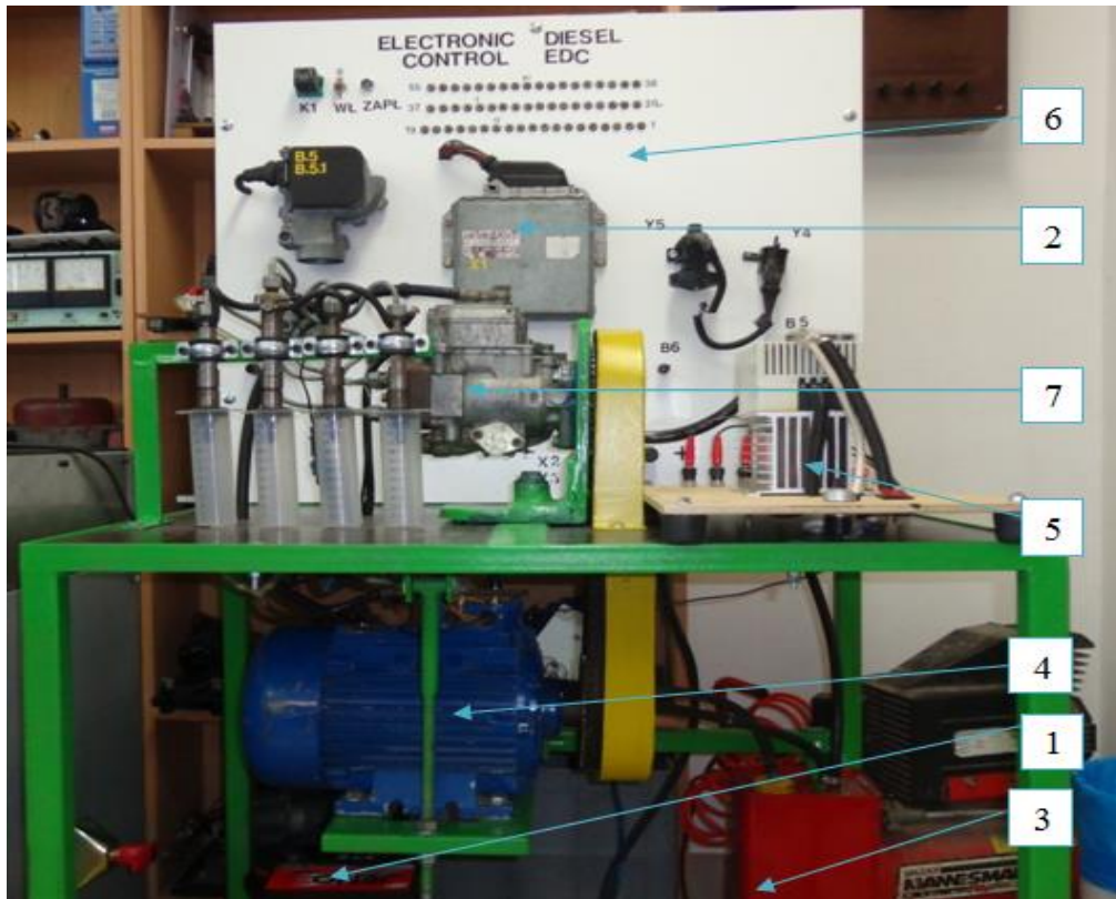
Fig.5. Test bench for testing the EDC system (1-battery, 2-controller engine, 3-fuel tank, 4-pump drive motor, 5- speed control system, 6- elements of the electronic control, 7-injection pump and fuel injectors)
