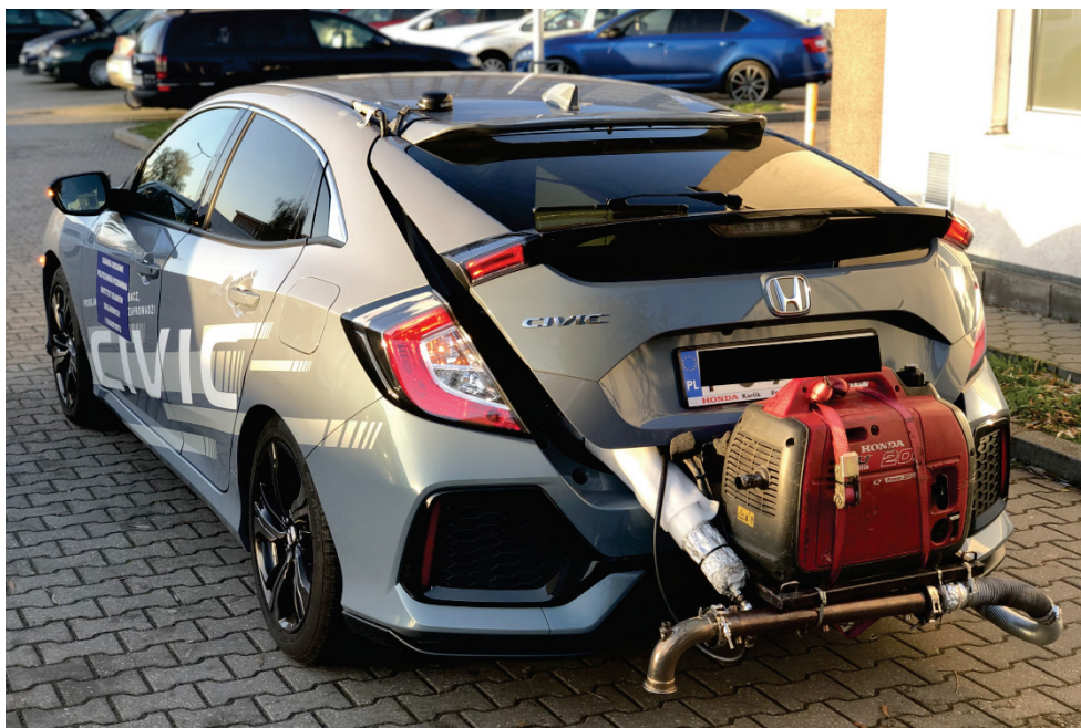
Fig. 1. View of the examined vehicle equipped with PEMS analyzers
