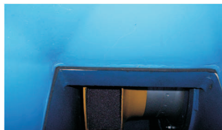
Figure 4. The smooth housing which was used for testing rotors with artificial roughness.
