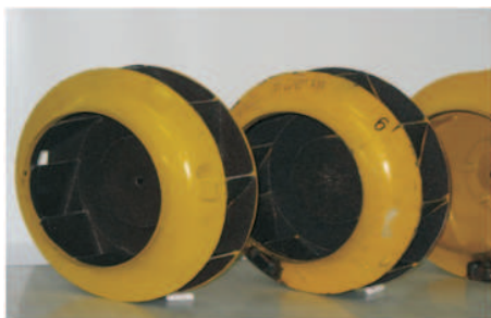
Figure 3. On the foreground the rotor with P40 sandpaper is show, second one is with P80 sandpaper, last one is smooth.
