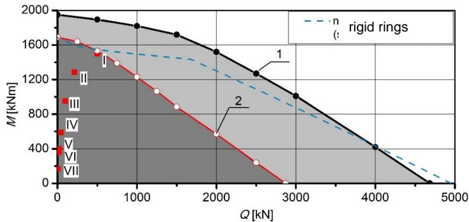
Fig. 8. Characteristics of the bearing capacity with marked work points of the mobile crane (1 - the catalog capacity taking into account the flexibility of the bearing rings, 2 - bearing capacity of the bearing installed in the crane at the angle of rotation of the body  $\theta = 45^\circ$ )
