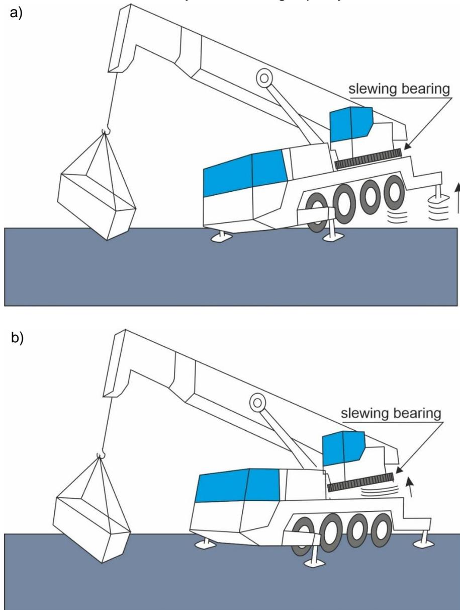
Fig. 2. Loss of crane boom stability as a result of carrying too much load (a) and damage to the slewing ring bearing (b)
