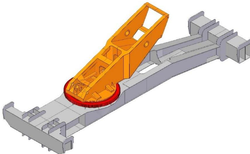
Fig. 6. Geometric model of the analyzed mobile crane
