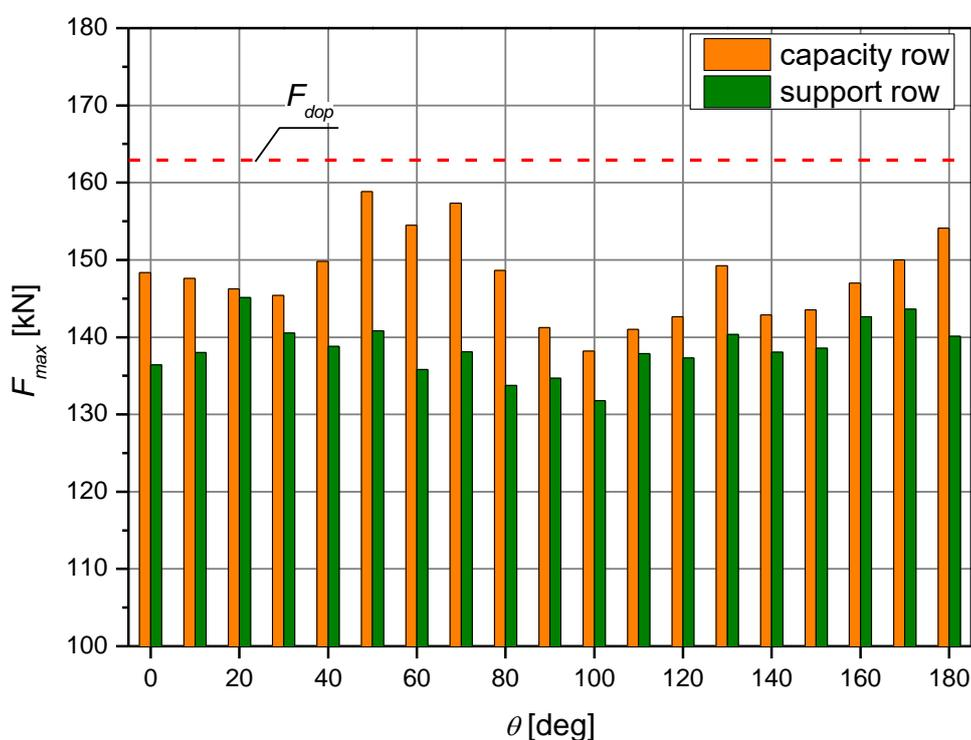
Fig. 10. Maximum loads on the rolling parts at different positions of the body (angle  $\theta$ ) in a crane carrying a load of 50 tons at a length of 3 m
