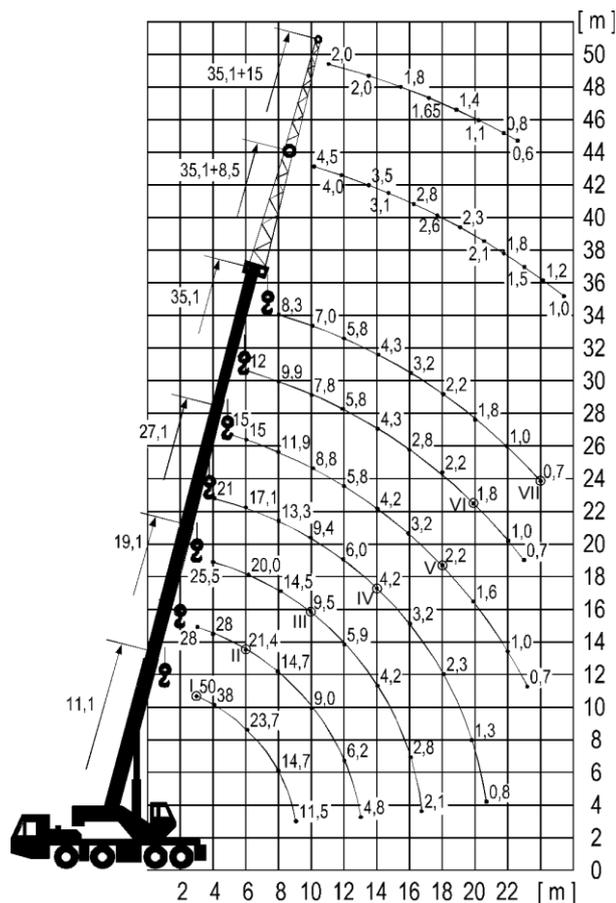
Fig. 5. Crane load characteristics
