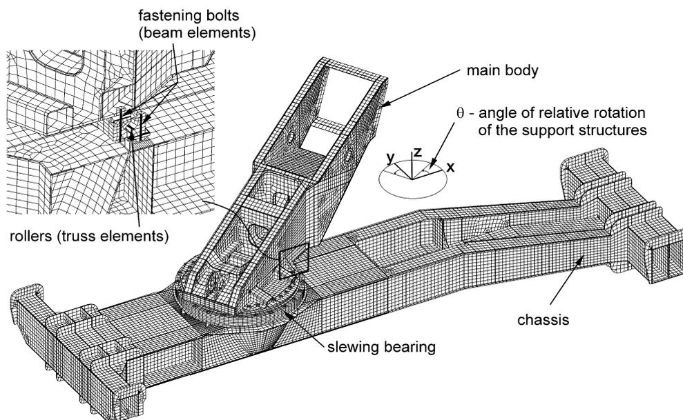
Fig. 7. FEM model of the analyzed mobile crane
