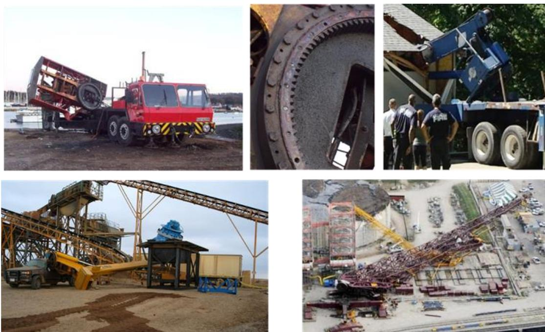
Fig. 1. Examples of catastrophes caused by damage to slewing bearings in cranes
