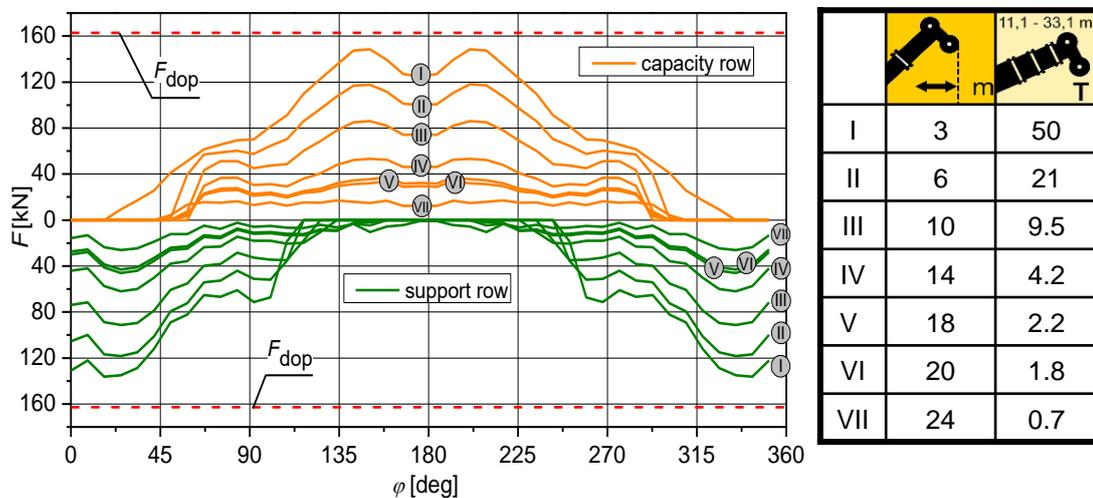
Fig. 9. The distribution of the internal load in the bearing of a mobile crane at different operating points of the crane for the angle of rotation of the body  $\theta = 0^\circ$
