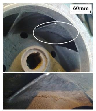
Fig. 3. Cavitation damage of the rotor disk located near the intake edge of the blades. The magnified area shows a typical, rough surface area of cavitation erosion [16]
