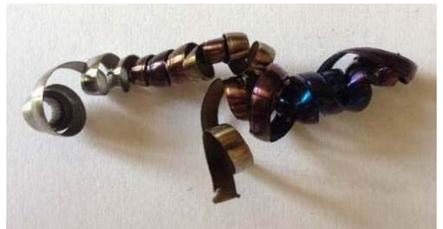
Fig. 10. Chip coloured due to cutting temperature
