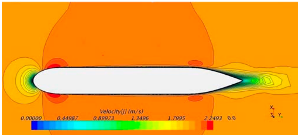
Figure 16. Velocity distribution around the hull (drift angle = 0^\circ , V = 2 m/s)
