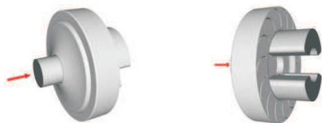
Figure 3. The three-dimensional computational domain of the blower aggregate BA0.
