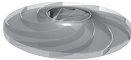
Figure 4. The three-dimensional computational domain of the impeller of the blower aggregate BA0 .
