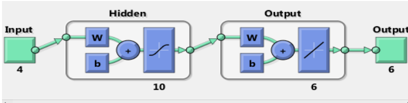
Fig. 1. Neural Network architecture for all mechanical properties
