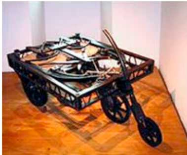
Figure 1. Self-propelled vehicle built according to the design of Leonardo da Vinci (Porathe, 2016)
