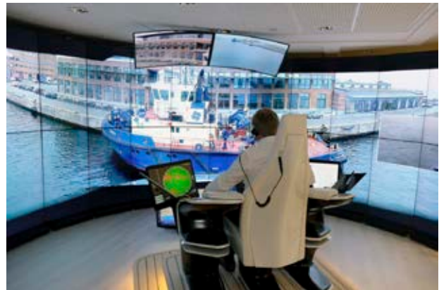
Figure 9. Remote maneuvering of the 28-meter tugboat Svitzer Hermod in the Copenhagen port in 2017 (Kongsberg, 2017)
