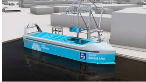
Figure 8. Project of the first unmanned container ship, in which 100% of the electricity is from the Norwegian transport company Yara (IMO, 2018b)
