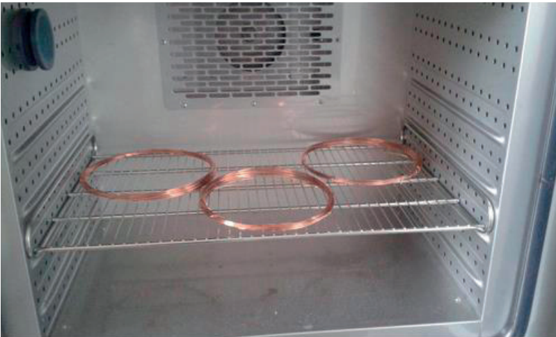
Fig. 6. Wires during moisturizing in an climatic chamber
