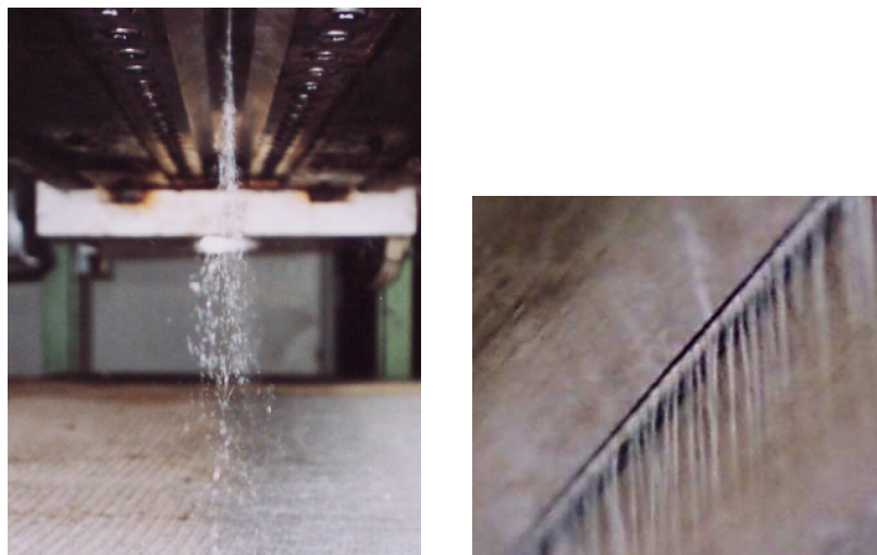
Fig. 2. Polymer stream flowing out of the spinning beam
