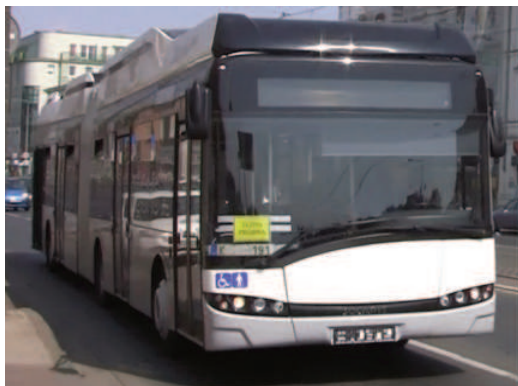
Fig. 2. Bus with a length of 18 m with a series hybrid drive system
