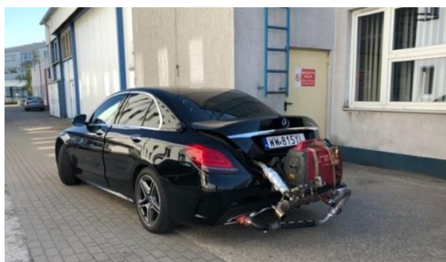
Fig. 3. Test vehicle – Mercedes-Benz W205 equipped with a spark-ignition engine with EQ Boost
