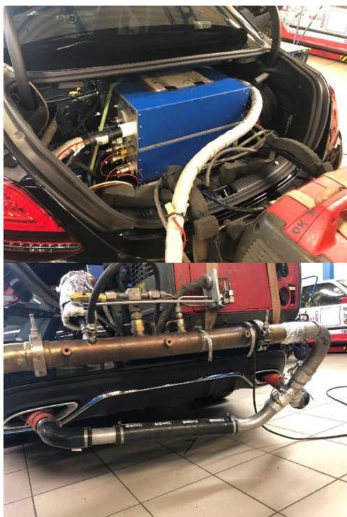
Fig. 5. Measurement equipment used for tests in real traffic conditions
