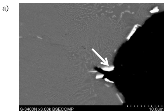
Fig. 6. The weld's microstructure at rupture line (a) and EDS spectra of marked precipitate (b)
