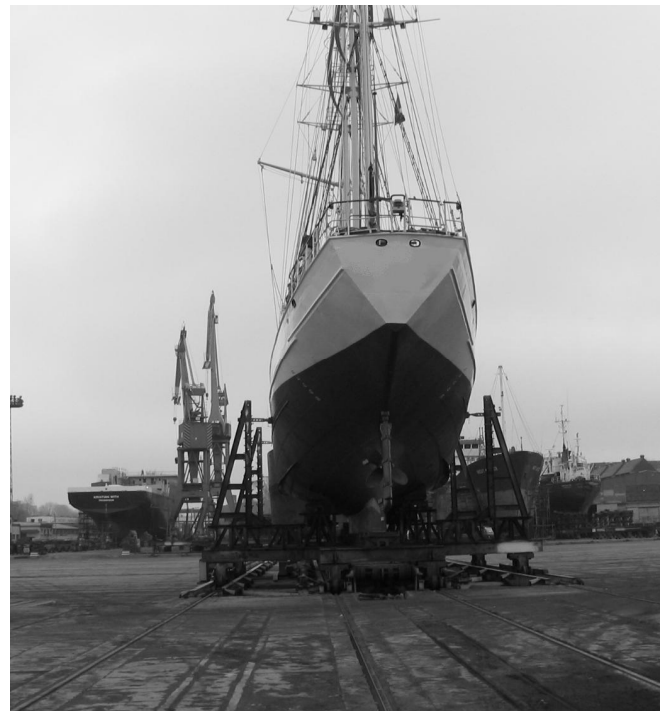
Figure 4. The ship during transportation from the traverser to the repair post R7
