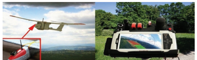
Fig. 5. Proposed concept in application to UAV; observation camera on UAV (left) and operator's console view (own elaboration)
