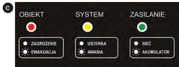
Fig. 3. WiSeNe MONIT – on-line subsystem: a) installation scheme, b) sample of the measuring device attached to the structure, c) the indicators on the front panel of the central unit (where: obiekt – object, zasilanie – power, zagrożenie – threat, ewakuacja – evacuation, usterka – defect, awaria – failure, sieć – network, akumulator – battery)
