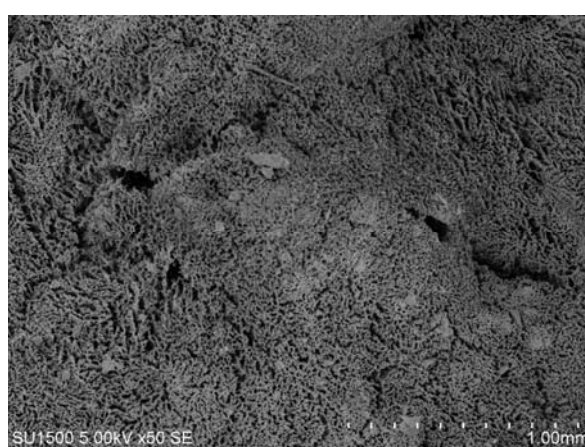
d. SEM of GCL with water content of 180% ( \times 50 )
