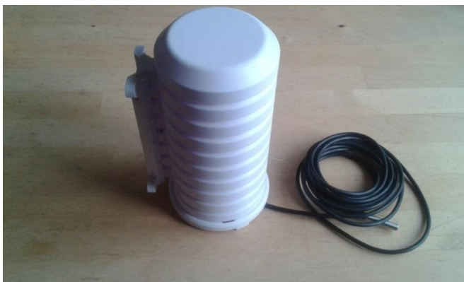
Fig. 6. The meteorological micro-station is placed in a protective casing and in a radiation shield
