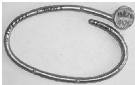
Fig. 7. Spiral test at 1420°C
