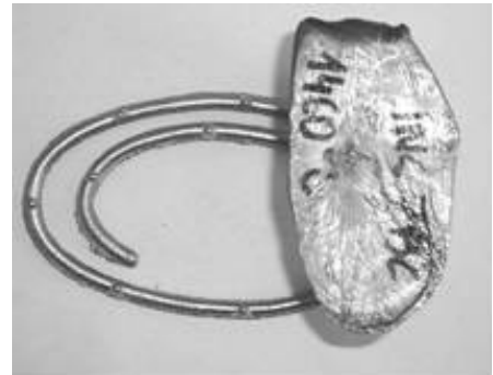
Fig. 8. Spiral test at 1460°C
