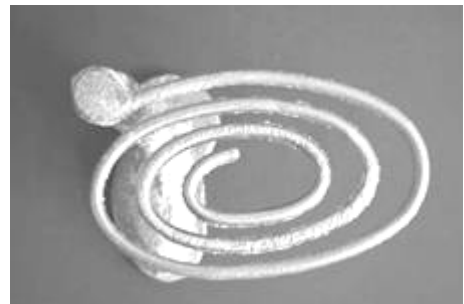
Fig. 10. Spiral test at 1600°C
