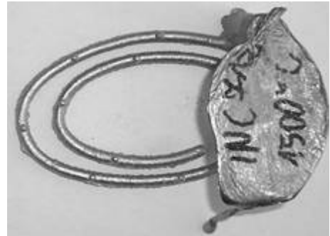
Fig. 9. Spiral test at 1500°C
