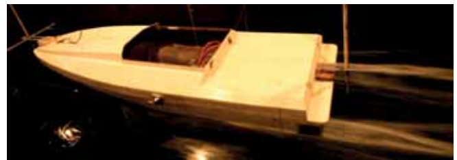
Fig. 8. High-speed navigation at 13 m/s without air jets
