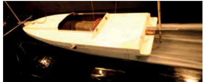
Fig. 7. High-speed navigation at 13 m/s with air jets
