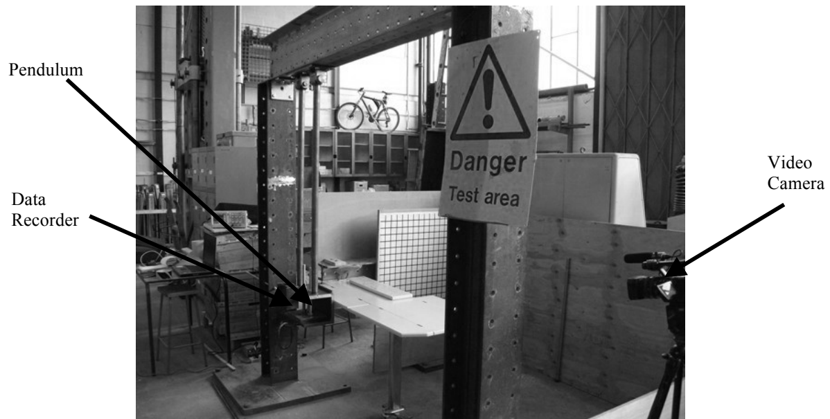
Fig. 7. Test Configuration (First Class TGV Table)
