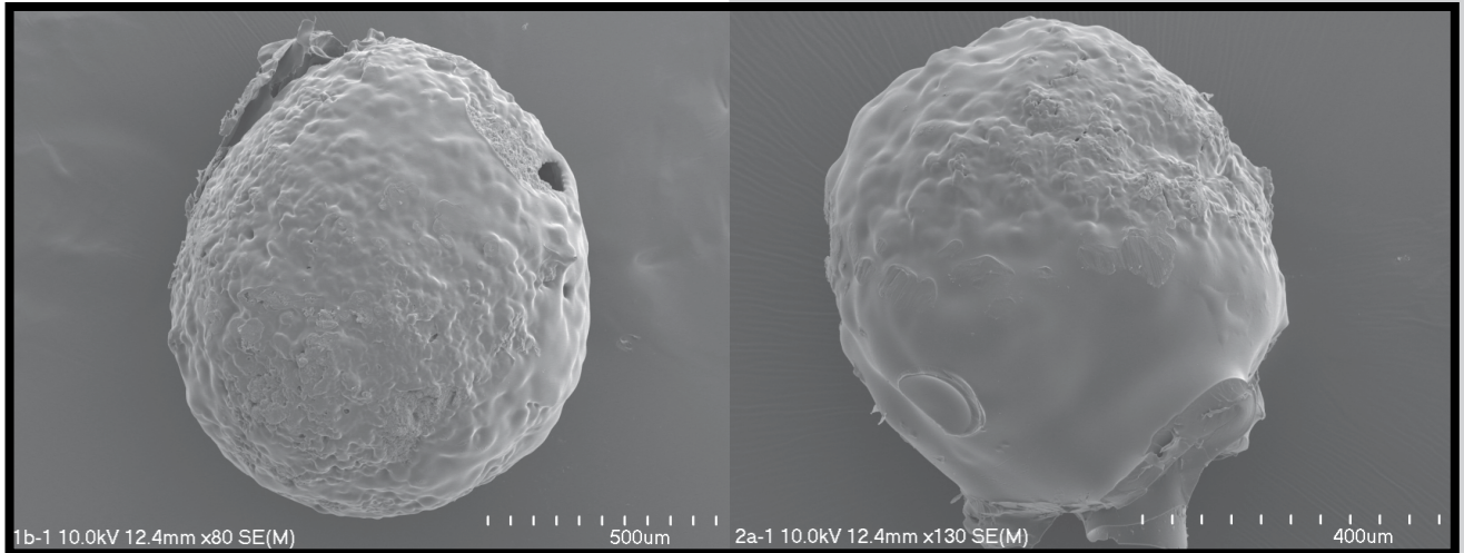
RYS. 4. Hydroksyapatytowe granule pokryte poli(D,L-laktydem). FIG. 4. Hydroxyapatite granules with poly(D,L-lactide) covering.
