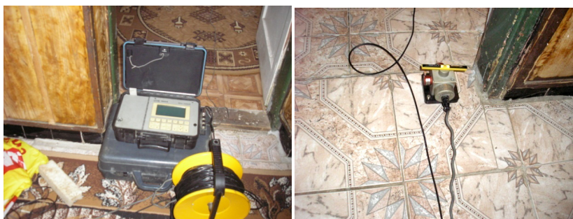
Fig. 4. Measuring position 2 – prior to entry into a house in the Kučín village; seismometer was placed on a foundation wall in front of the house.
