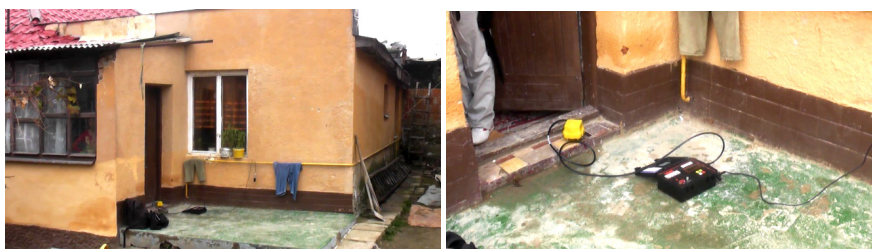
Fig. 3. Measuring position 1– residential house No. 44 in the Kučín village; three–component seismometers from the American company Geospace at the entrance of a residential building.
