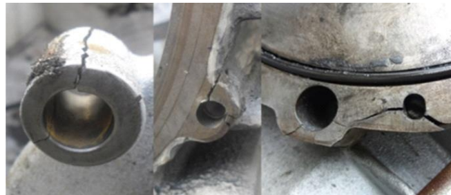
Figure 2. Examples of damaged pumps due to vane malfunction [1]
