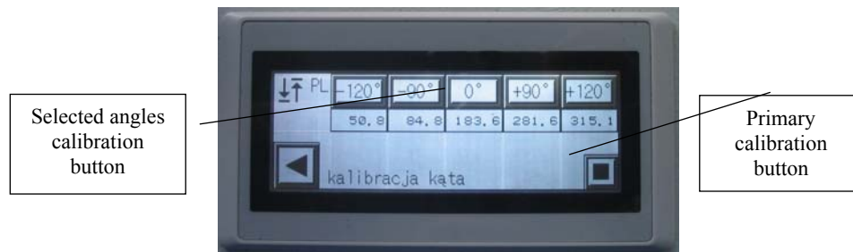
Fig. 6. Angle measurement track calibration screen \alpha
