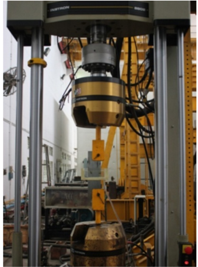
Fig. 2. Set-up of CFCG experiment on an ESE(T) specimen
